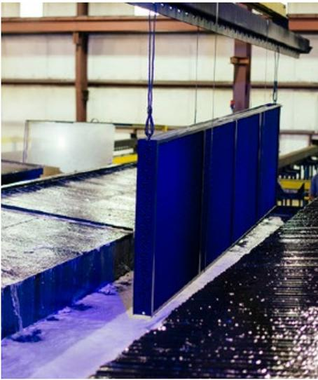
***ElectroFin E-Coat is specifically formulated to lengthen equipment service life by four to five times and have less than 1% impact on the thermal efficiency of the coils it protects.***
